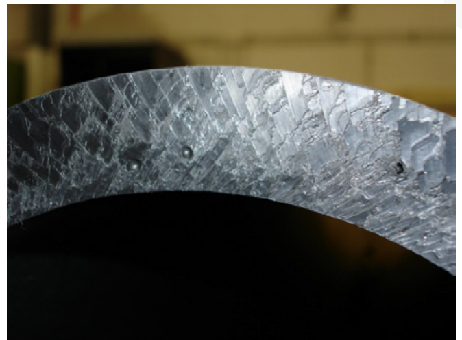
Figure 2. Example of pipe extruded from a resin with elevated moisture content resulting in uneven inner pipe wall (top) and holes in the pipe wall (bottom).
