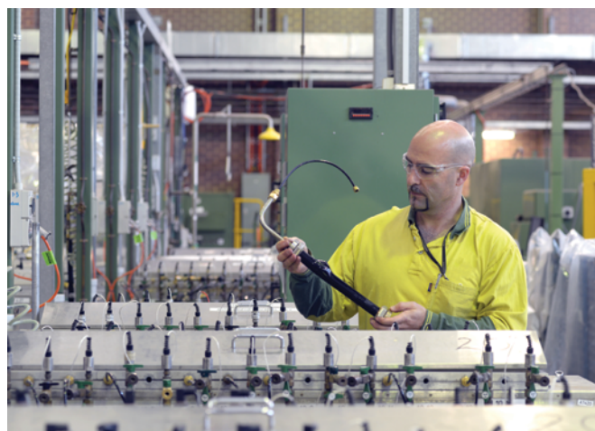
Pressure data collection at elevated temperatures in the Qenos Technical Centre, Altona
