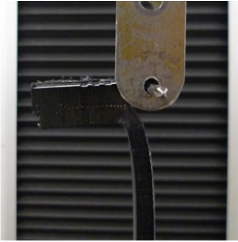
Figure 1. Peel test setup as per ISO 13954
